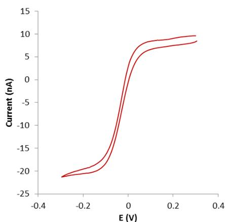
Cyclic voltammogram for 1 mM ferrocenylmethyl alcohol in 0.1 M  $\text{H}_2\text{SO}_4$  at a thin-film **gold** microelectrode array (ED-mSE-10-Au).  $v = 10 \text{ mV/s}$ .
