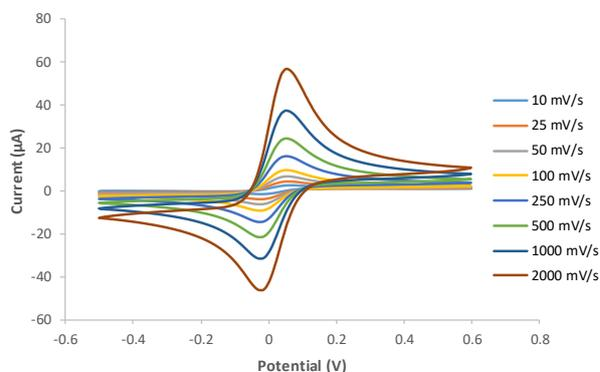
Cyclic voltammograms for 1 mM ferrocene methanol in 0.1 M  $H_2SO_4$  using different **scan rates** at a thick-film carbon electrode (ED-S1PE-C10).
