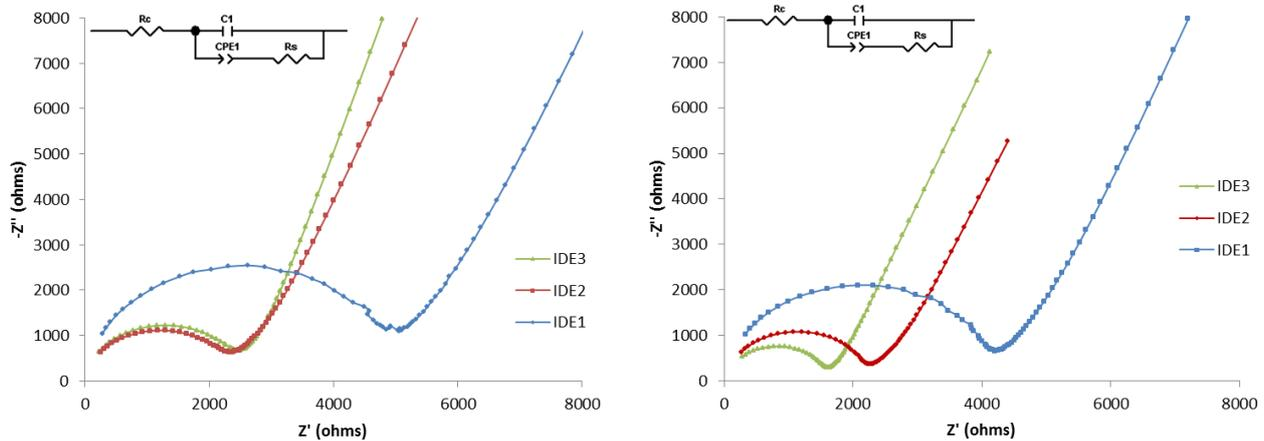
Nyquist plots using **different** gold and platinum thin-film **interdigitated electrodes** in a low conductivity NaCl solution (6.0 mS/cm). Frequencies range: 500 kHz – 100 Hz,  $V_{p-p} = 25$  mV. **Inset:** equivalent electric circuit.
