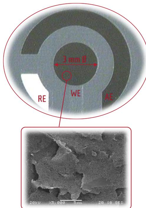
**Thick-film graphene-based electrodes** have a very low electrical resistance with a good scratch resistance for using in a wide variety of applications, including the development of low-cost *chemical-sensors* and *bio-sensors* for field analysis.
