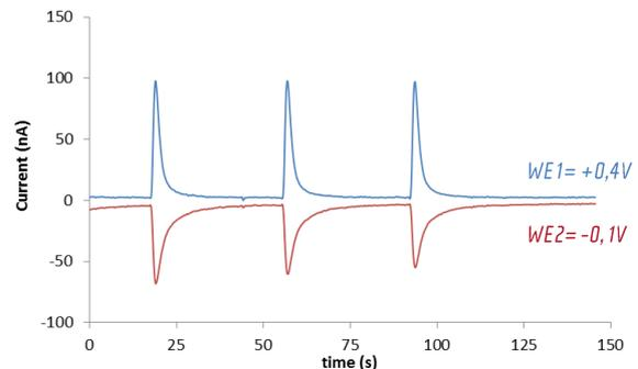
Amperometric response for  $1 \cdot 10^{-5}$  M pAP in a FIA system using a thin-layer microfluidic interdigitated array platinum electrode (TL-IDA1-Pt) applying same and different detection potentials.
