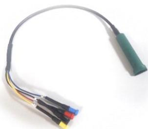
The **SPE-CABLE connector** (*Ref. ED-SPE-CABLE*) provides an interface between the **thick-film electrodes** (up to four contact pads) with the potentiostat, enabling the use of microvolume (20 – 50  $\mu\text{L}$  sample drops) or dipping into a solution. The cable ends are available with 2-mm female or male bananas.
