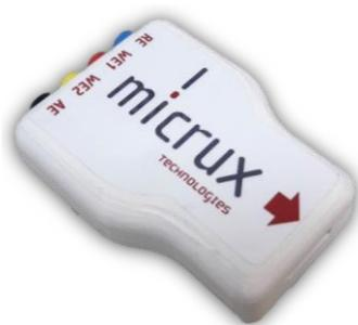
The small **BOX connector** (*Ref. ED-SPE-BOX*) provides an interface between the **thick-film electrodes** (up to four contact pads) with any kind of potentiostat, enabling the use of microvolume (20 – 50  $\mu\text{L}$  sample drops). The interface ends are available with 2-mm female bananas.
