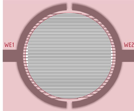
Different interdigitated electrode (IDE) designs are available in platinum or gold.
