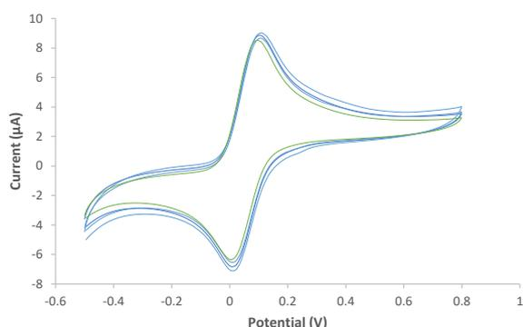
Cyclic voltammograms for 1 mM ferrocene methanol in 0.1 M H<sub>2</sub>SO<sub>4</sub> at the **same** thick-film graphene electrode.  $v = 50$  mV/s
