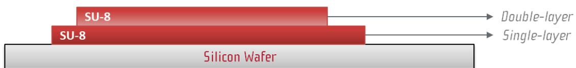
Silicon wafer could be cut on smaller rectangular pieces in order to get individual masters. Other technical features can be fulfilled under request.
