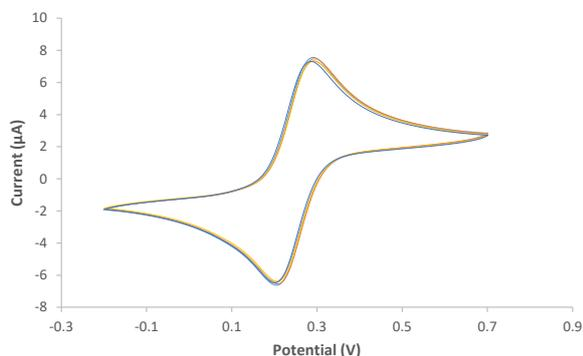
Cyclic voltammograms for 1 mM  $K_4Fe(CN)_6$  in 0.1 M  $H_2SO_4$  at different thick-film gold electrodes.
