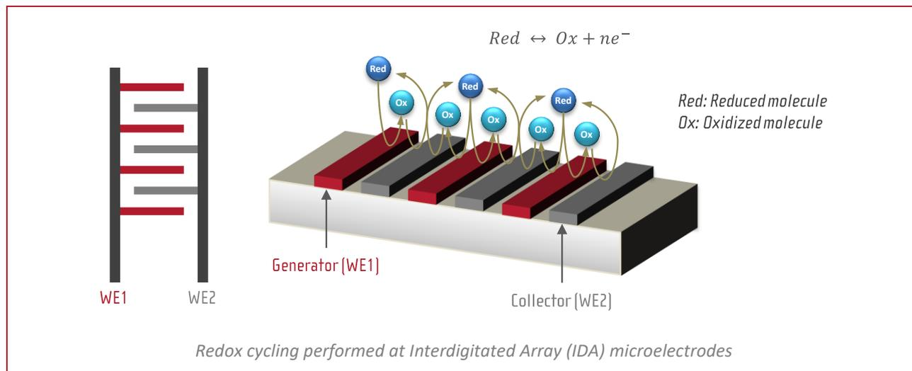
IDA microelectrode designs (*width and gap*) are going to affect the number of *redox cycling* as well as the *collection efficiency*.
