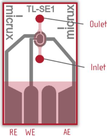
» Microfluidic Electrochemical cell
