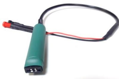
The **IDE-CABLE connector** (*Ref. ED-IDE-CABLE*) provides an interface between the **thin-film IDE electrodes** (IDE - two contact pads) with the potentiostat, enabling the use of microvolume (2 – 10  $\mu\text{L}$  sample drops) or dipping into a solution. The cable ends are available with 2-mm female or male bananas.
