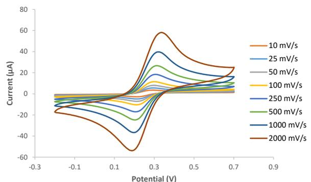
Cyclic voltammograms for 1 mM  $K_4Fe(CN)_6$  in 0.1 M  $H_2SO_4$  using different scan rates at a thick-film carbon electrode.
