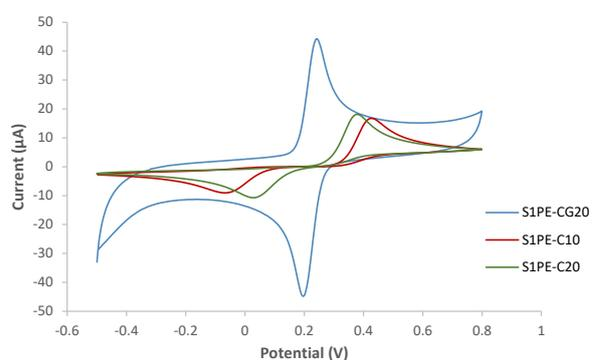
Cyclic voltammograms for 1 mM hydroquinone in 0.1M H<sub>2</sub>SO<sub>4</sub> at different thick-film carbon (ED-S1PE-C10 / ED-S1PE-C20) and activated **graphene**-based electrodes (ED-S1PE-CG20).  $v = 50$  mV/s.
