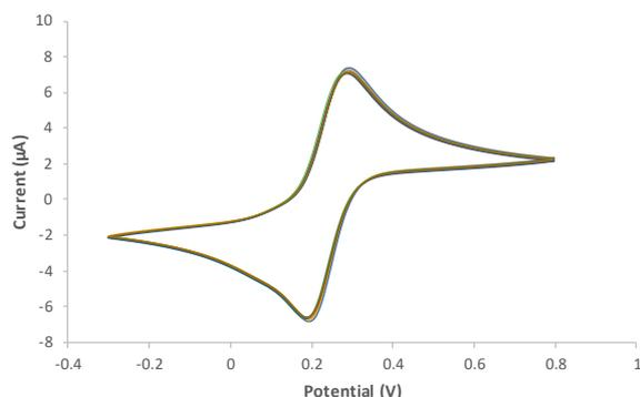
Successive cyclic voltammograms for 1 mM  $K_4Fe(CN)_6$  in 0.1 M  $H_2SO_4$  at the **same** thick-film carbon electrode (ED-S1PE-C10).  $v = 50$  mV/s,  $n = 10$ , **RSD = 2%**
