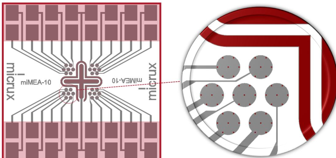
**Multi-iMEA chip** consists of four areas with seven sets of seven 10- $\mu$ m microhole arrays (28 individually addressable microelectrode arrays) with integrated reference and auxiliary electrodes in the center of the chip.
