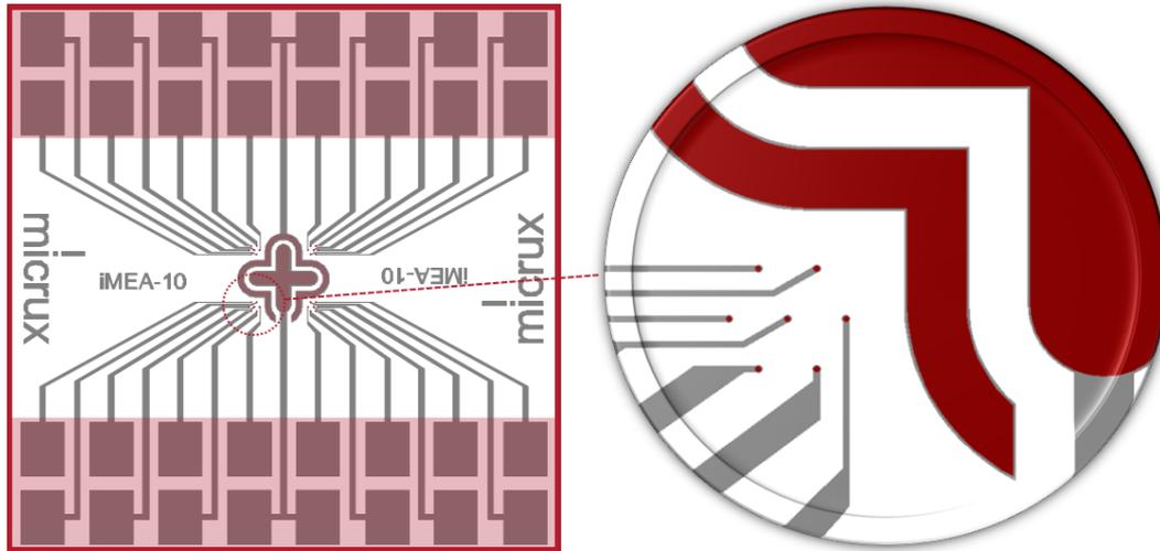
**iMEA chip** consists of four sets of seven 10- $\mu$ m microelectrodes (28 individually addressable microelectrodes) with integrated reference and auxiliary electrodes in the center of the chip.
