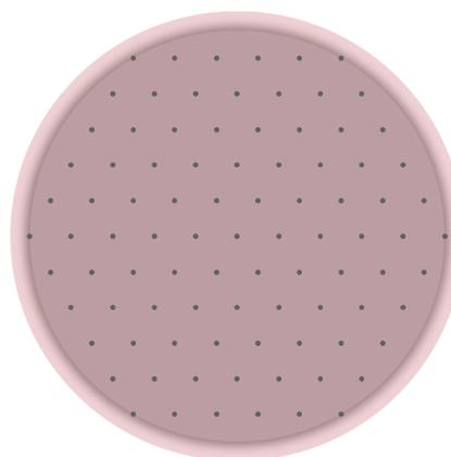
The working electrode (1 mm diameter) is based on a metal surface coated with SU-8 resin in which is defined a **microholes array** with **honeycomb structure**.
